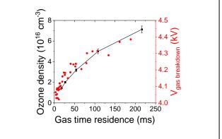
Fig. 1. Gas breakdown voltage and ozone density for different gas time residence
